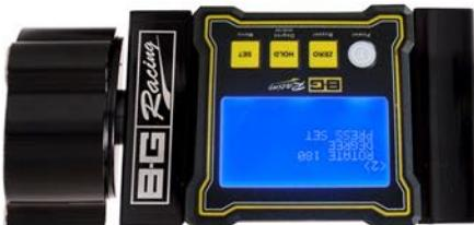
3. Once the buzzer has stopped LCD will display "<3> CALIBRATION HORIZONTAL PRESS SET". Stand the unit horizontal and press the "SET" button again and the buzzer will beep.
