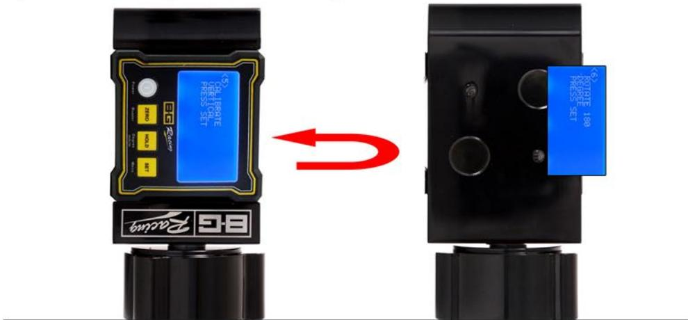
7. The unit is now calibrated, and the LCD will display the main menu, using the "ZERO" button & "HOLD" button to toggle, select "BACK" and press "SET" button to return to the measuring display.
